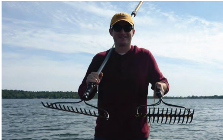
Figure 3. Two different rake samplers used during the Clearwater Lake surveys. [left] Fixed head sampler. [right] Double headed throw rake.
